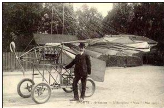
A postcard with Vuia and his airplane (weight 250 kg, surface 14 m 2 and a 20 PH engine)
